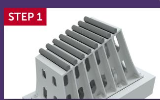
After the outer plates are removed, **hydraulic jacks will be installed** between the old, roller bearings.
