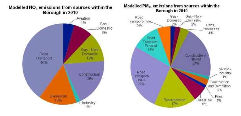
The charts below and overleaf focussing on transport emissions, show the breakdown of emissions of  $NO_x$  and  $PM_{10}$  from different vehicle and fuel types. These show that emissions from diesel vehicles account for almost 90% of transport emissions of NOx and 90% of tail pipe emissions of  $PM_{10}$ . Additionally for  $PM_{10}$  the total emissions which include tyre and brake wear emissions are also estimated as these are now included in the latest inventory.
